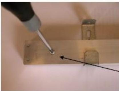
**VITE DI BLOCCAGGIO**
