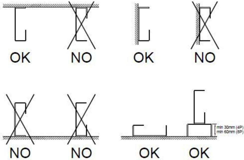
4.1 If you are suspending the busbar on Threaded rod, wire systems etc you must Install alternative hangers on opposite sides as shown below. This is to ensure the busbar cannot be displaced from the bracket if the busbar is damaged or hit for example.
