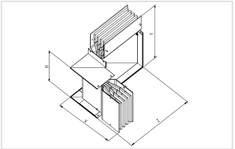
**TRIPLO ANGOLO TIPO Z3 • "Z" TRIPLE ELBOWS - TYPES Z3**
