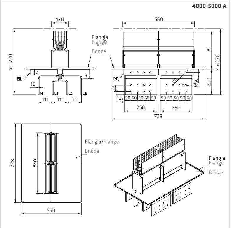
TESTATA TERMINALE CON ANGOLO • TERMINAL HEADER WITH ELBOW
